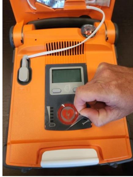
Figure 2: Remove the protective film by lifting it from its edge, if present.
